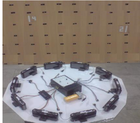
Fig. 10: Calibration of stereo panorama system using a test-field
