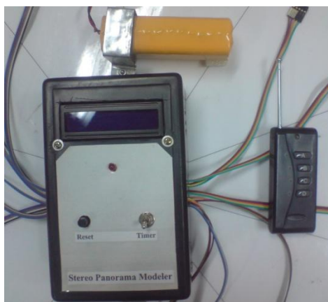
Fig. 9: The electronic control unit, battery and remote controller of the stereo Panorama Modeler
